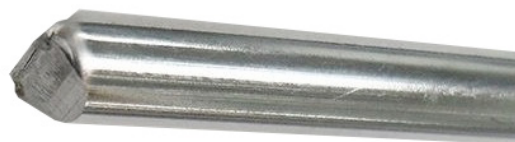
Rod cut by standard pinching-type rod cutter
